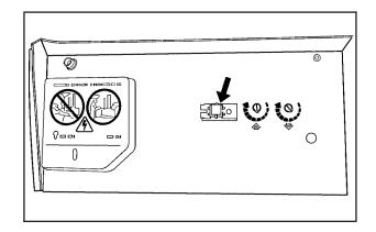
After Steps 1 through 5 have been completed, locate inside the garage the garage door opener receiver (motor-head unit). Locate the "Learn" or "Smart" button. The name and color of the button may vary by manufacturer.
